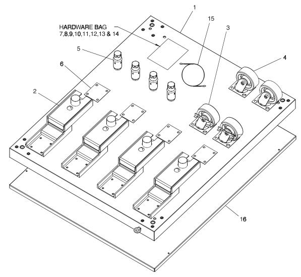
Figure 2-4. Model PS540 Triple Oven Option Base with Outriggers and Top
